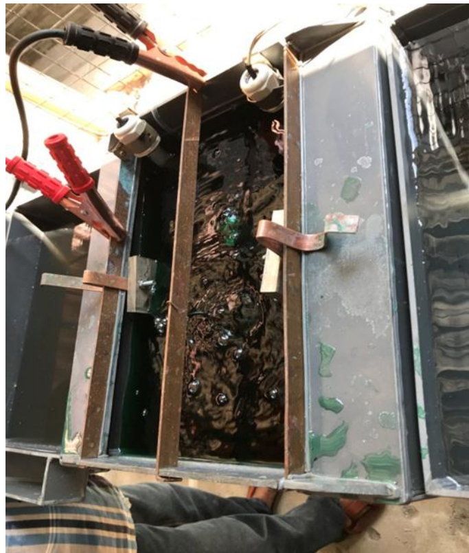
Gambar 3.36. Proses copper kilap plating
