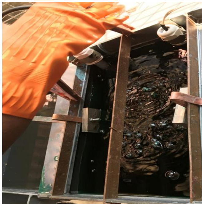
Gambar 3.34. Proses nikel kilap plating
