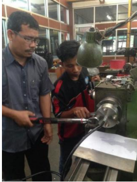
(a) Tightening force measurement.
