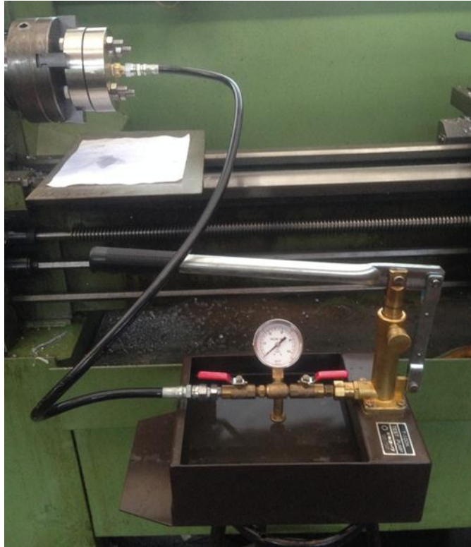
Gambar 3.13. Water pressure test
